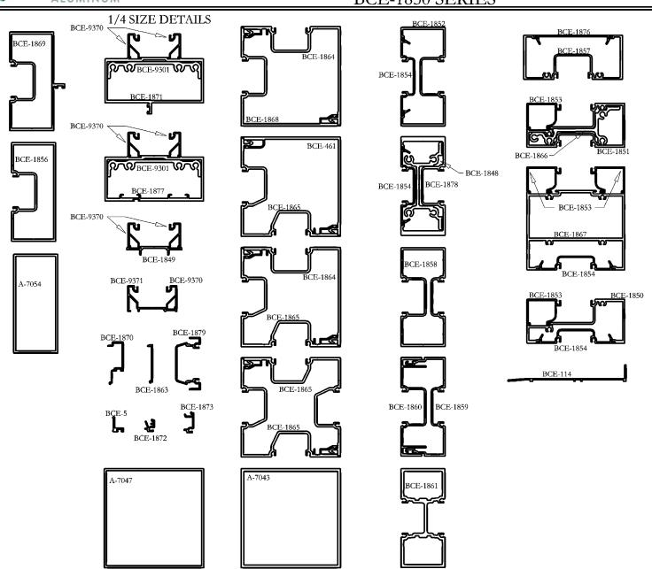
THIS SYSTEM IS DESIGNED TO BE ASSEMBLED WITH #12 SCREWS.
