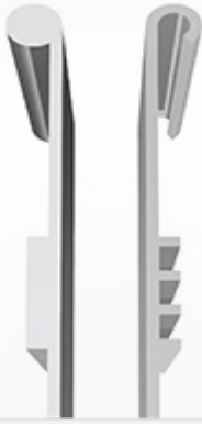
Part on left features varying wall thickness. On right, the same part with uniform thickness.
