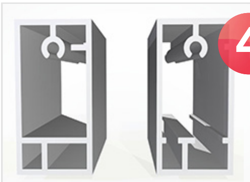
The part on the right is corrected to remove cavities and does not reduce overall strength of the part.
