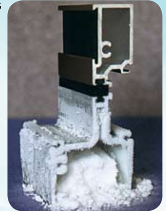
Pour & Debridged sample subjected to dry ice with a surface temperature of -109° F demonstrating the effectiveness of the thermal break properties.
